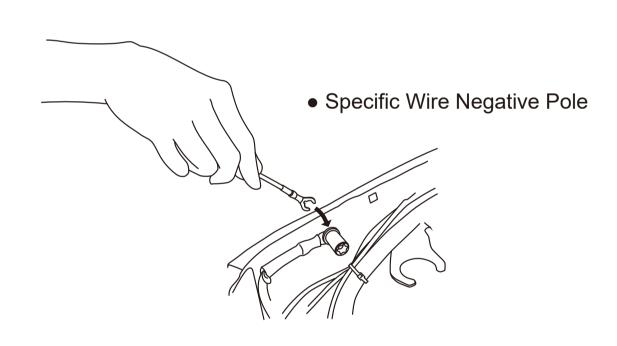
• Pay attention to whether negative pole is conductive, connecting the negative terminal to the vehicle's chassis or frame.
