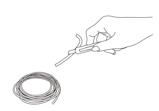
• Please pay attention: Do not fold or press the pipe when installing, otherwise it will damage the pipe structure. Cut the pipe with a knife, scissors will deform the pipe.
