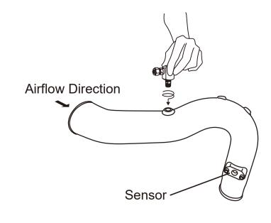
Please note that turbo pipes with methanol hole are for specific vehicles, please choose correct model. When drilling the hole, please note that it must be in front of the sensor.
