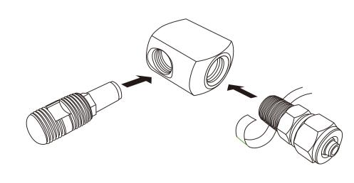
Please pay attention when wrapping the anti-leakage tape, it needs to be in the opposite direction to the screw thread.
