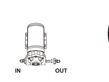
Please pay attention to IN / OUT • Waterproof gaskets need to be placed in the inlet/outlet holes of pump.
