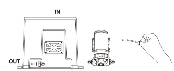
Please pay attention to OUT. Waterproof gasket need to be placed in the outlet hole of methanol / water tank. Use screws to secure the pump onto the methanol/water tank.
